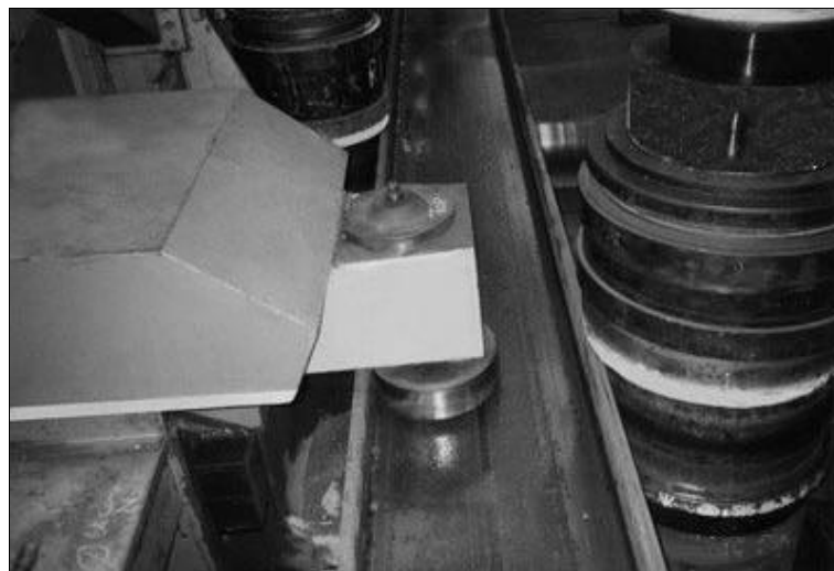
Figure 3.4 Bending of an open section showing additional rolls to prevent web buckling
